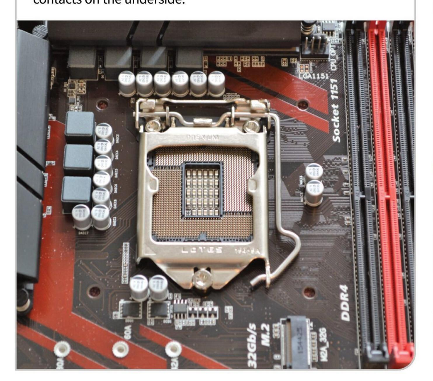
The arrow shows you which way the chip sits in the socket (arrow to arrow). Intel processors also have a small indentation on each edge, which further helps you to line it up in the socket. Holding the CPU carefully by the edges, lower it it into place in the socket. Ensure it is seated correctly, with the arrows and the notches lined up and in place.
