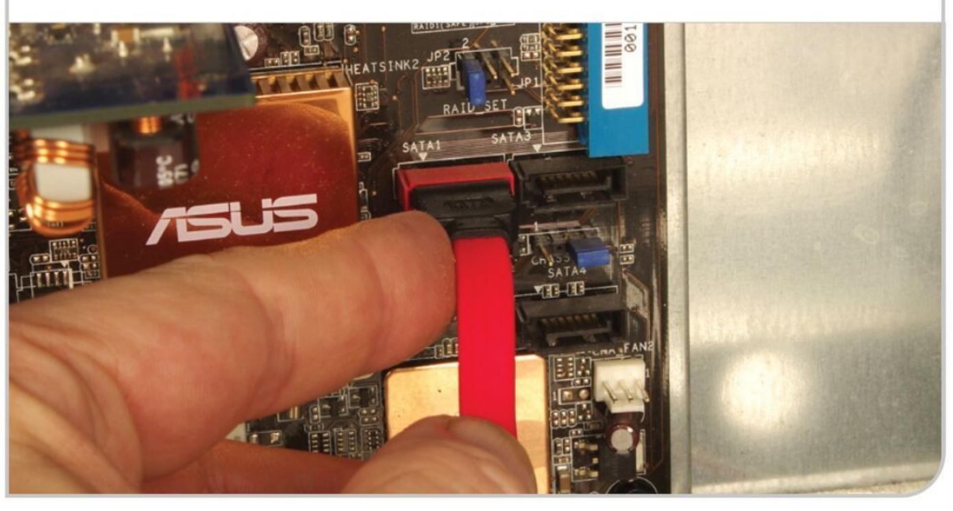
Plug the other end of the SATA data cable into the socket on the SSD. Push it in all the way until it clicks. It can only go in one way, so you can't connect it the wrong way round. Push firmly but don't force it.
