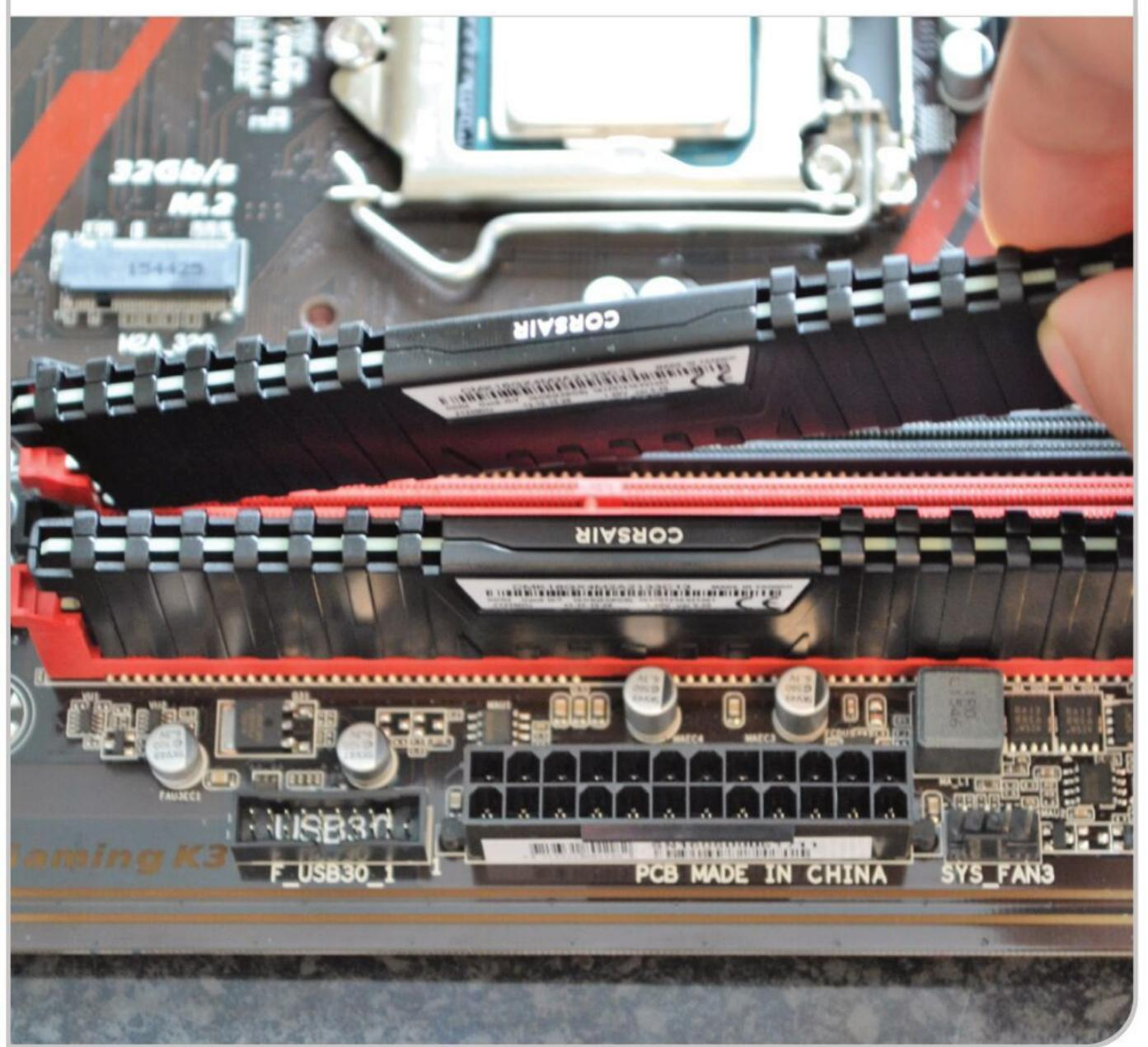
Memory modules have an offset notch in the row of connectors on the bottom. This will correspond with a divider in the motherboard memory socket, ensuring that you can't insert the DIMM the wrong way around. The memory socket will also usually have a hinged clip at each end that needs to be pressed down and away from the socket.
