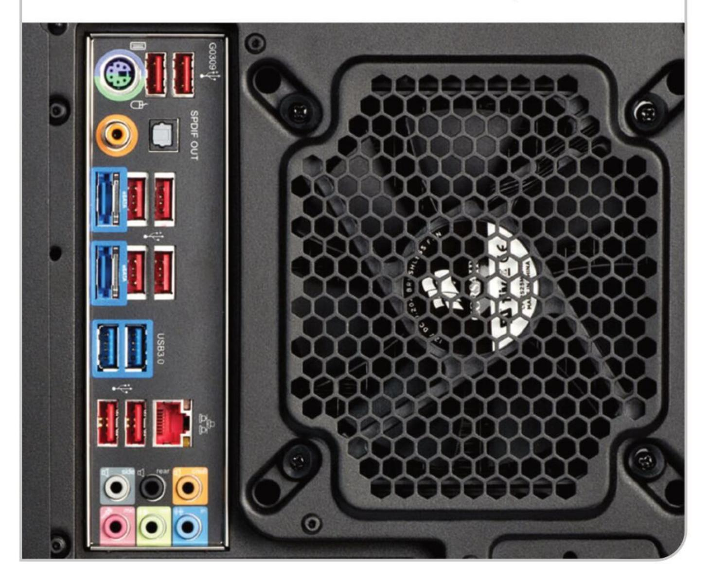
If you're planning on using an Ethernet cable for networking, connect it to the Ethernet port on the rear of your PC. The other end of the cable can be connected to your router or Wi-Fi bridge. If you have an external Wi-Fi aerial, you will need to plug this into one of the USB ports on the rear panel of the tower.
