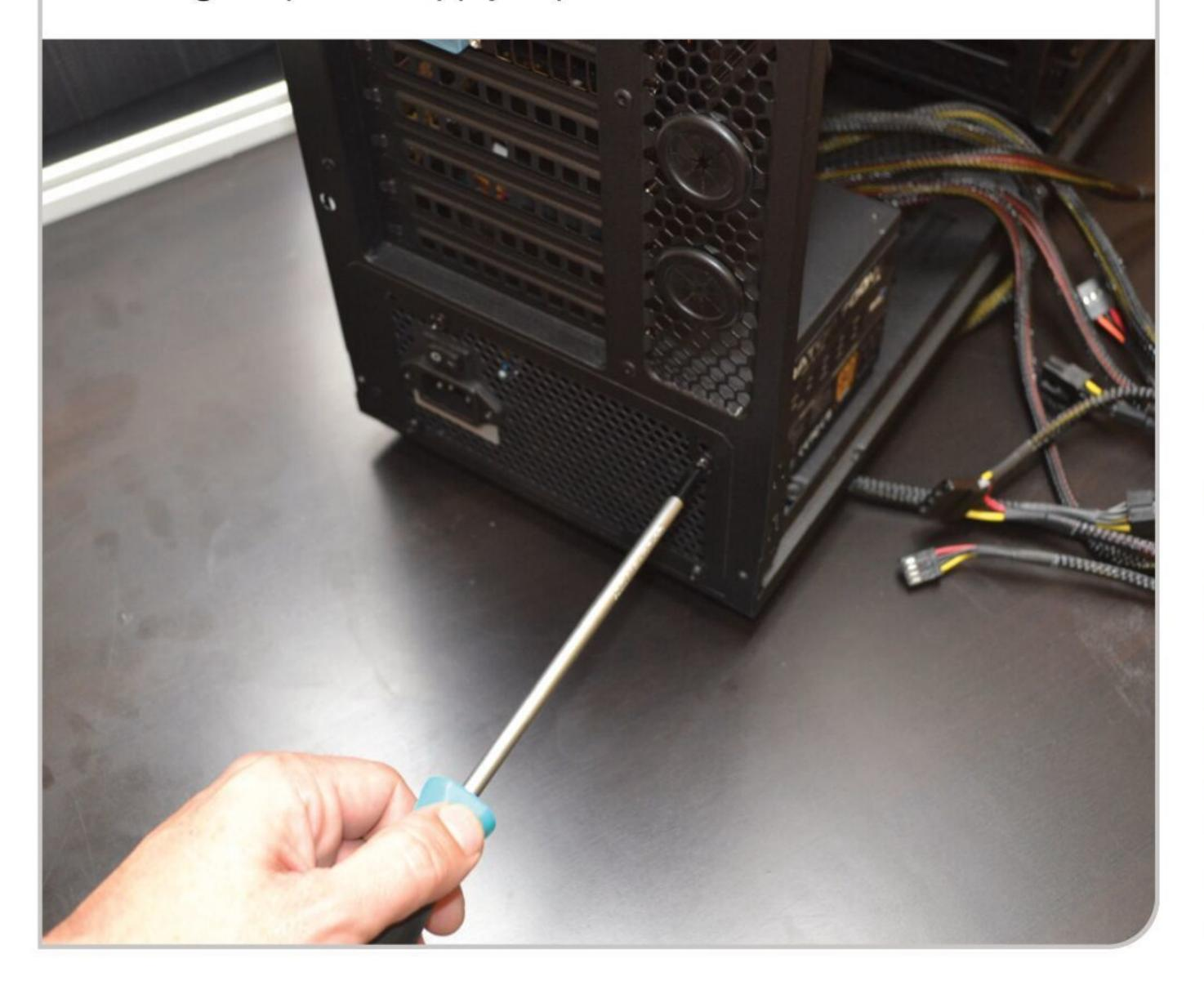
STEP 5 If your case has cable management holes in the back of the chassis, you can start feeding cables through at the bottom of the case. Work out how many of the different PSU cables you need: probably a 4+4-pin, the main 20+4-pin, the PCIe 6-pin and a couple of SATA connections and tidy up the rest. If you are using a modular PSU, store the excess cables safely in the box.
