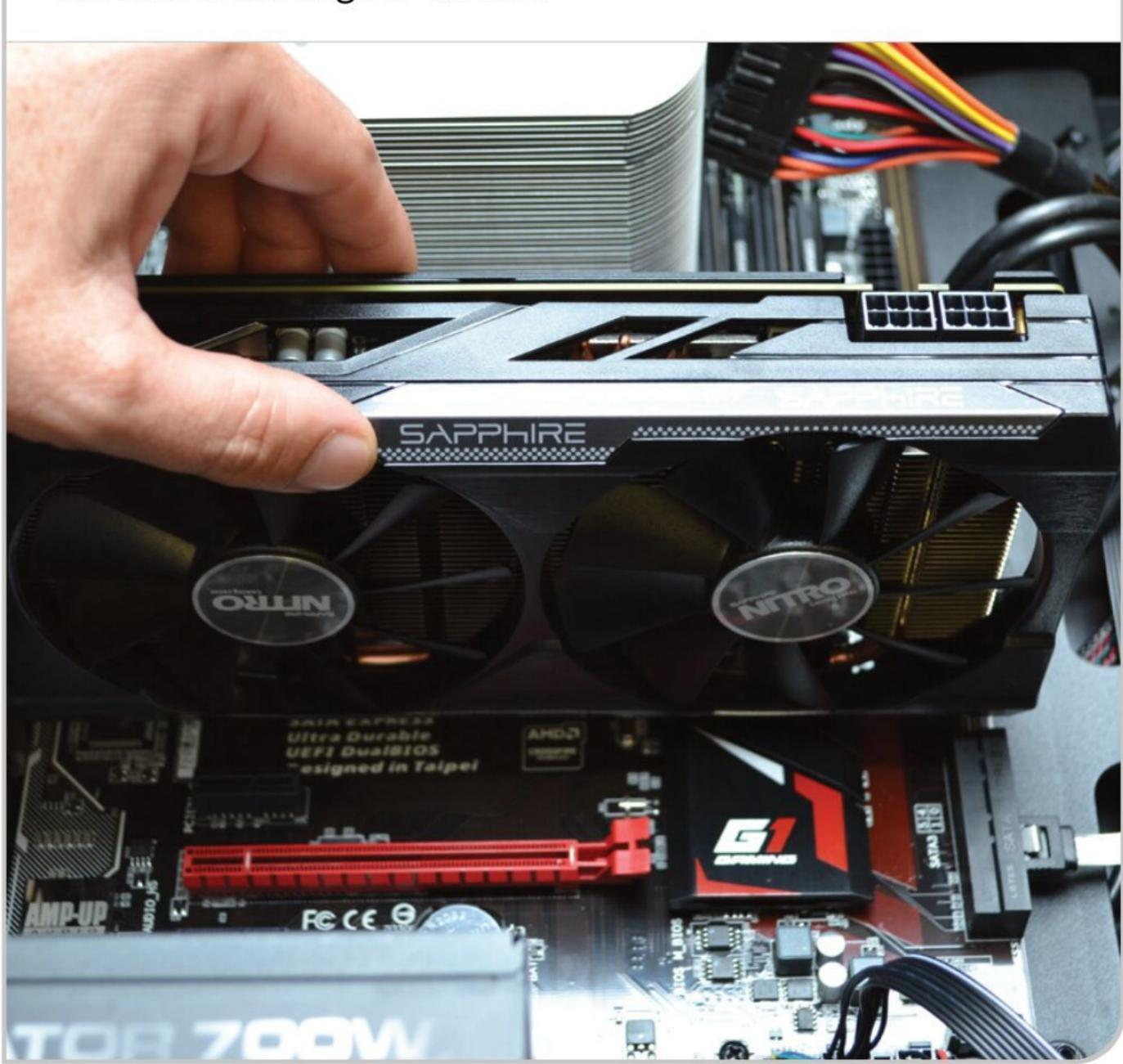
Many motherboards, especially gaming motherboards, will have a second PCIe socket. This allows you to run two graphics cards in SLI or Crossfire modes, assuming you have cards that are SLI or Crossfire compatible. The slots are normally spaced slightly apart to allow for improved airflow from the cards on-board fan but apart from this consideration, the above steps can just be repeated.
