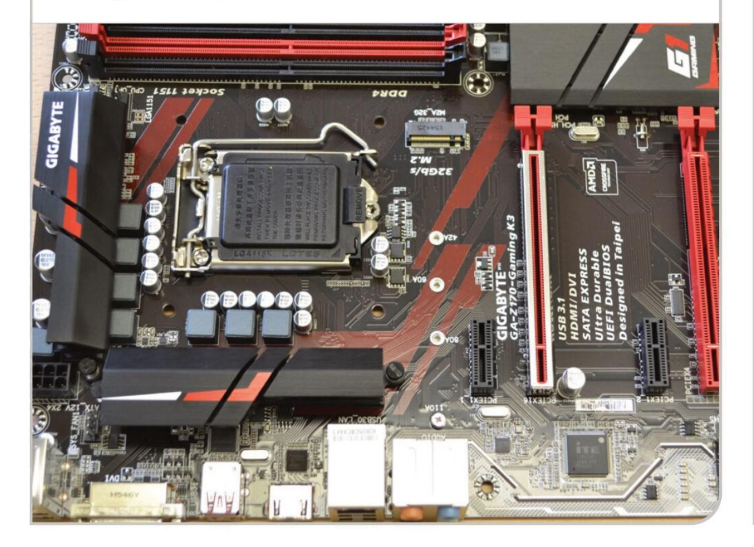
The process for fitting an AMD or Intel CPU is similar, but there are some physical differences between the two processor types, not least the arrangement of the contact pins. We are using an Intel Core i5 6600k CPU for our build and we will concentrate on that process. See further down the guide to see specific AMD CPU installation advice and precautions.
