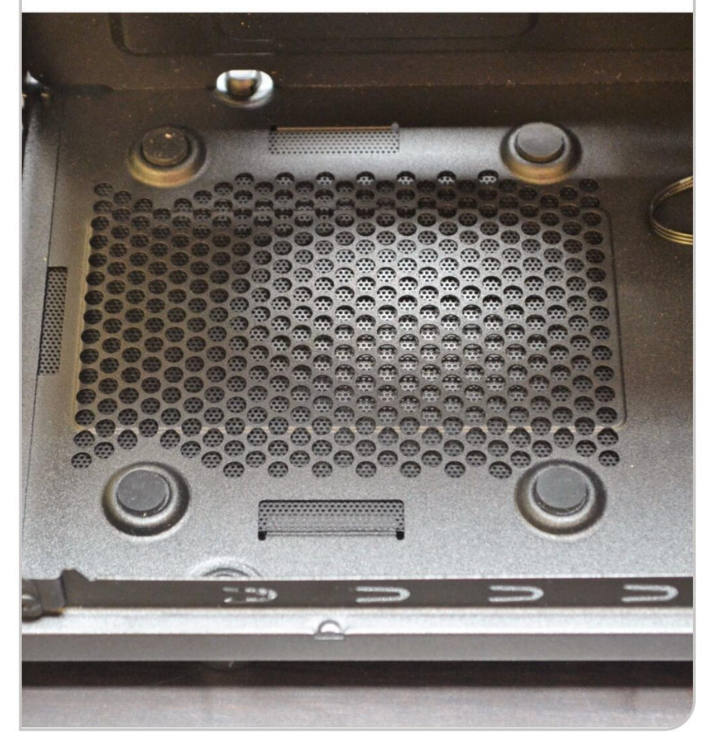
Position the PSU in the case, with the power socket facing out and the cables facing in to the case. The screw holes on the power supply will line up with holes around the edge of the PSU opening. The screws should have been supplied with the PSU but if not, standard case screws will do the job. There should be at least four screws holding the power supply in place.
