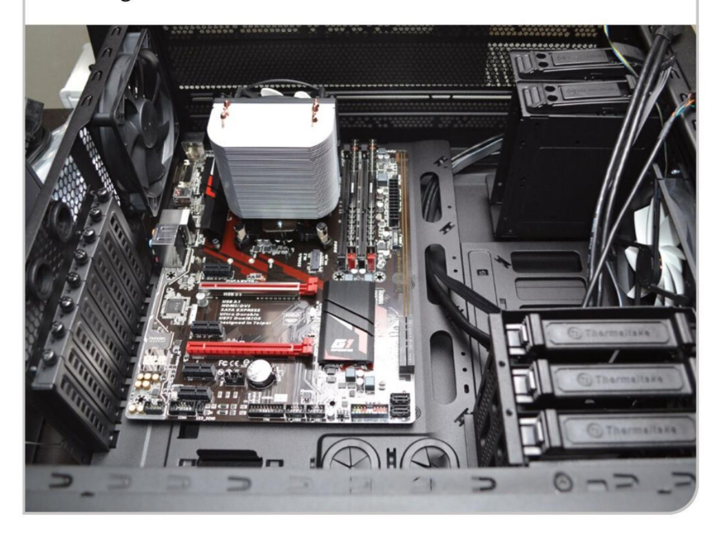
Once you have worked out where things need to connect, you can use the cable management holes to thread the cables around the back of the case to where they need to go. Most of the connections can only attach one way. They will either have guides on the plastic connector housing or one of the pins on the connector will be missing.
