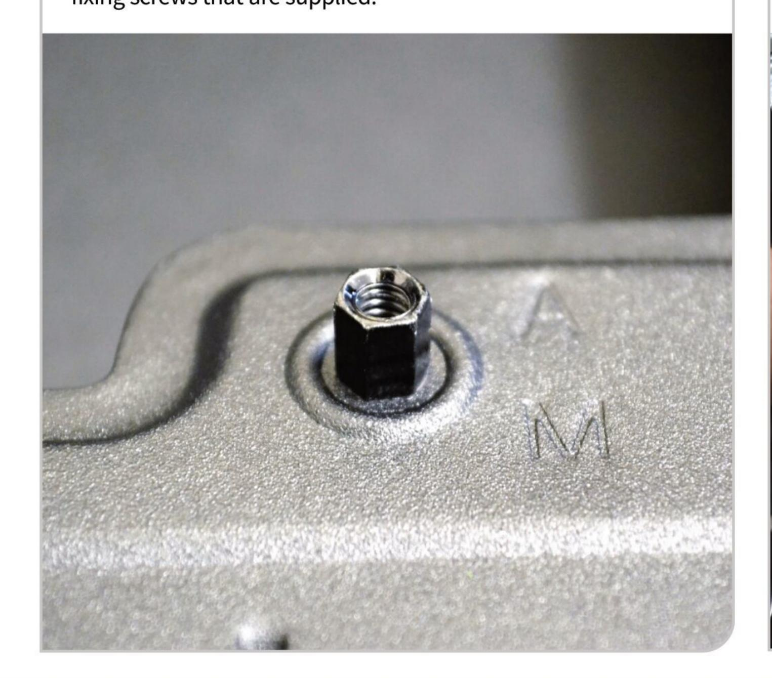
Carefully line up the back panel ports with the back plate holes, press the motherboard against the plate and screw one of the motherboard fixing screws into one of the holes to hold it in place. You can now insert screws into all of the other holes on the motherboard and tighten them carefully. You don't need to apply too much pressure when tightening the screws.
