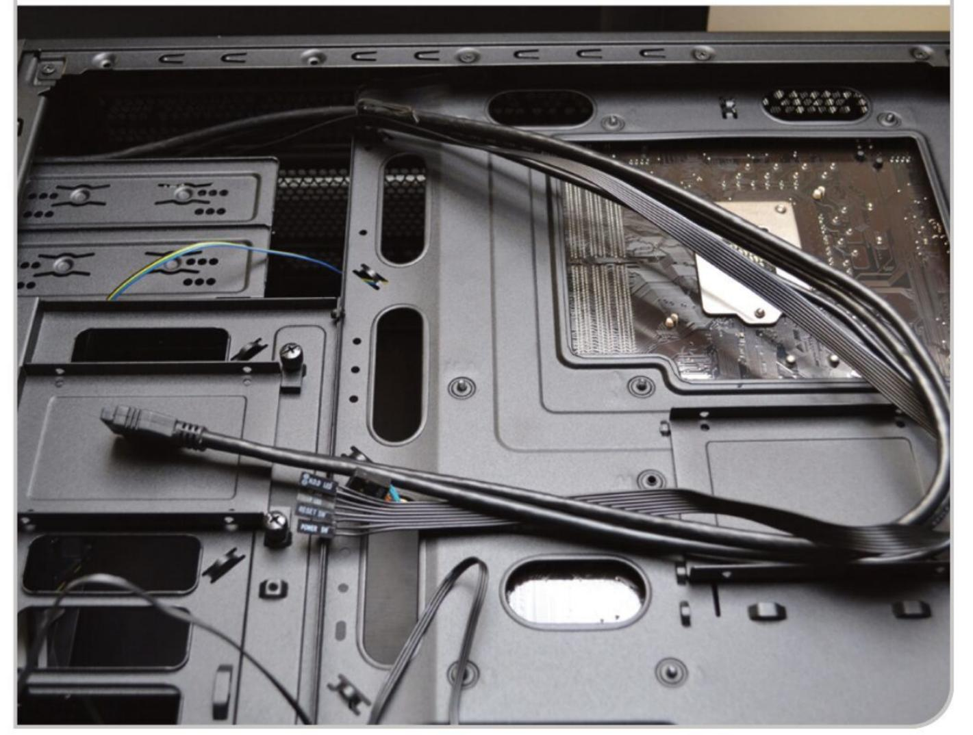
Apart from possibly the case fan connection, connections for front USB, audio in and out sockets and the power and reset switches are normally positioned along the bottom edge of the motherboard. Each connection socket will be labelled on the motherboard but this is sometimes hard to see. Check the motherboard manual if unsure.
