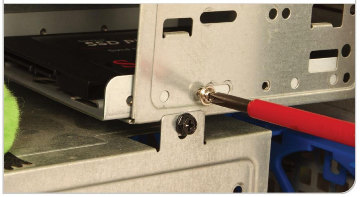
If you've already installed your SSD, open up the PC case again and disconnect the old hard drive. If you don't plan on using the HHD again you can remove it. You'll need a small cross-head screwdriver to undo the screws holding the drive into the bay.
