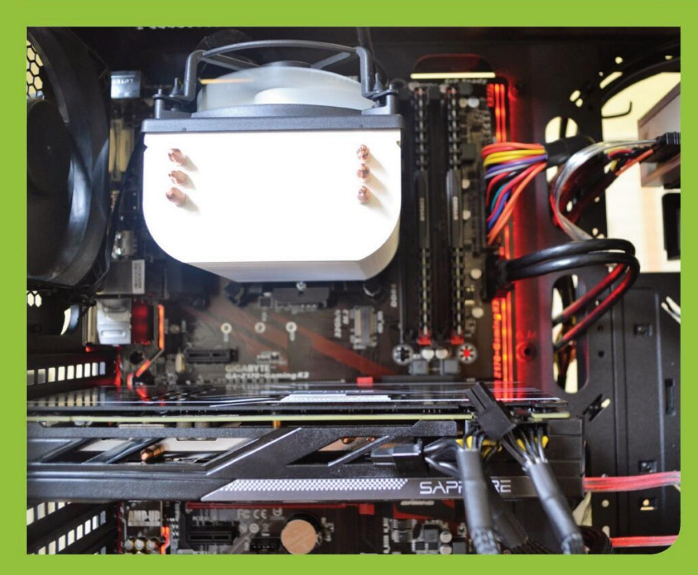
In this situation, the system enters a power-up power-down repeating cycle, where it looks like it is booting but then hangs and restarts. This is potentially a major concern as it can be a sign that the motherboard is defective. If it's not the motherboard, then make sure the CPU and memory are properly seated.
