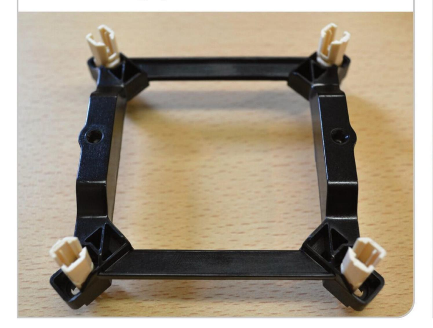
Carefully position the mounting plate on to the STEP 2 motherboard, lining up the pegs with the holes on the board, before pressing them through. This will see the mounting plate held loosely in position. You now need to push a pin into the mounting peg in each of the corners, pressing firmly down until you feel a slight click. The mounting peg is now held firmly in place.
