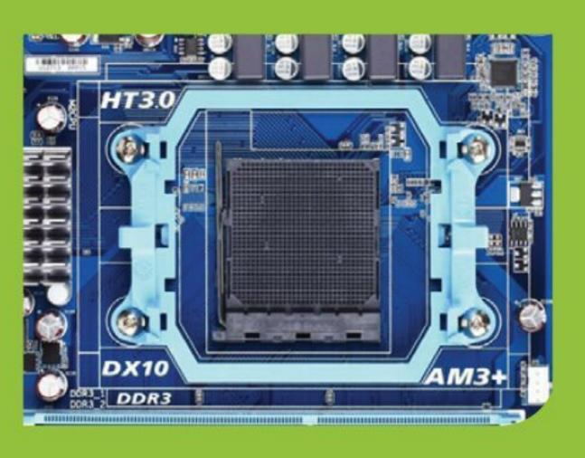
STEP 3 With your motherboard carefully placed on a flat surface, a thin sheet of anti-static foam beneath the motherboard will help to stop it moving or being damaged, and positioned so that the locking lever on the CPU socket is pointing towards you, carefully take the processor out of its box. Only ever touch the CPU on the sides, never touch the contacts on the underside.
