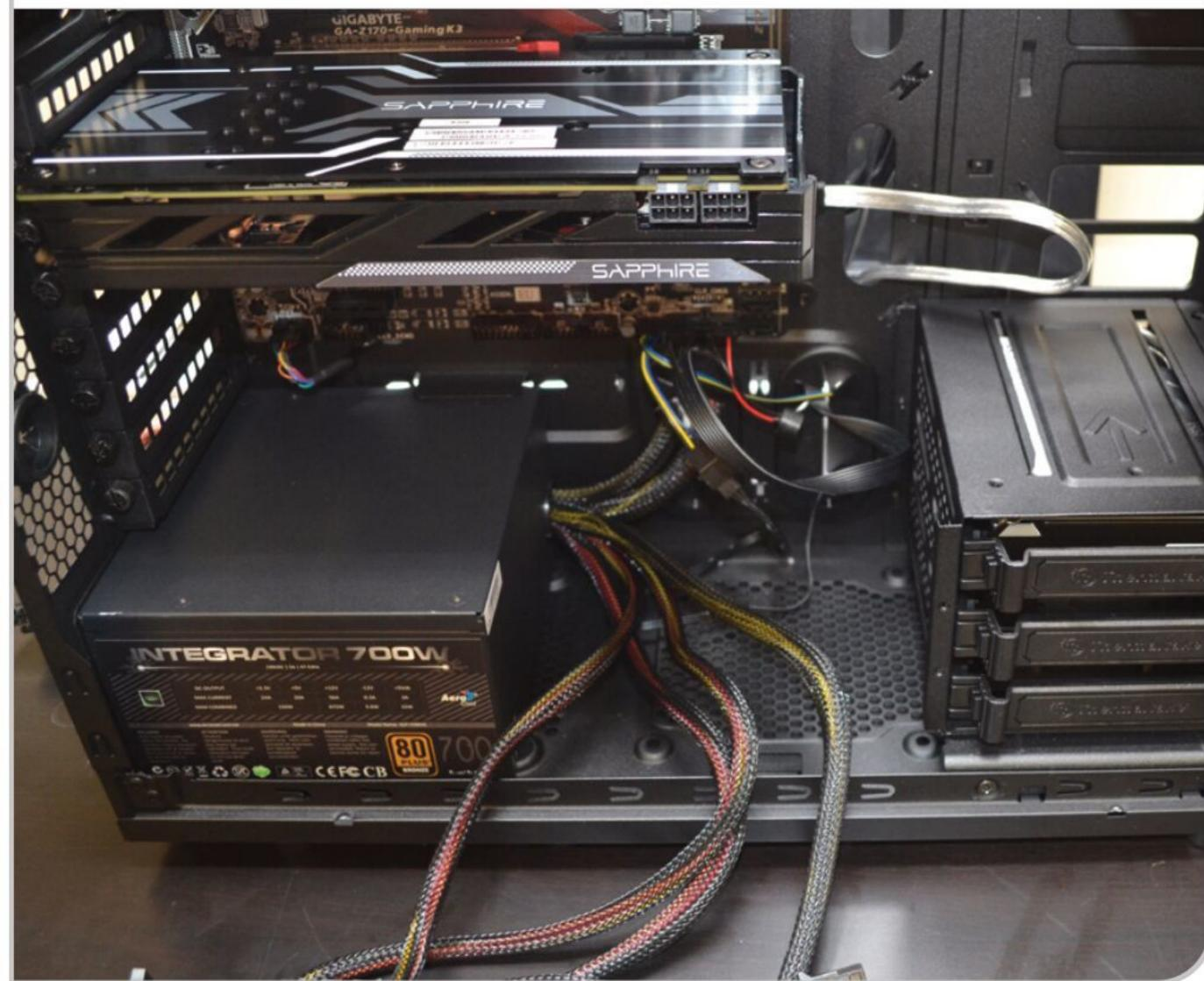
The bundle of wires coming out of the PSU may be tied or held together. Untie them and straighten them out. Some full tower cases are huge inside, and it is not unusual that the cables of the PSU aren't long enough to reach the 12v or 24-pin connection ports. If this is a problem for you and your PSU didn't come with extensions, you will have to purchase the ones you need.
