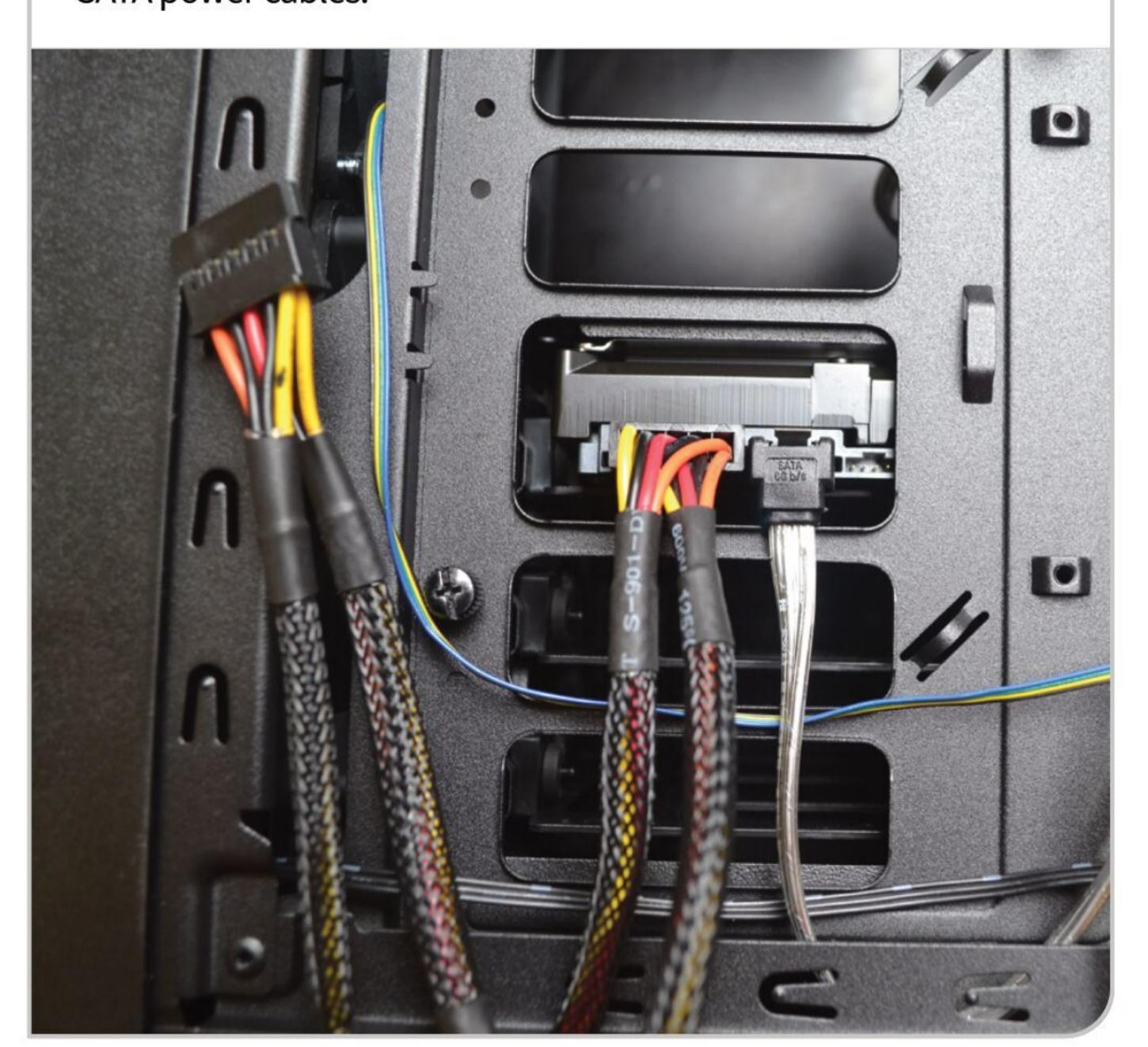
Keep airflow in mind and don't cover any case fans or coolers with a cable if at all possible. The Component placement within a system is also important. Drives, graphics cards and other expansion cards should be positioned in such a way that their cables, or the components themselves, don't interfere with one another. Don't be afraid to move a component if needed.
