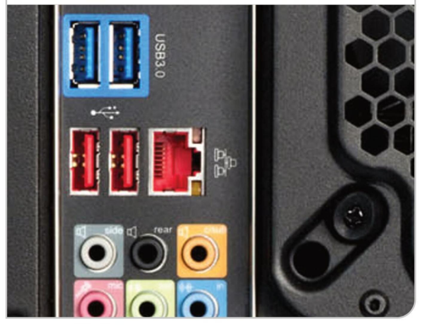
If you have a set of speakers that you'd like to use, connect them now. If you're simply connecting a pair of stereo speakers, connect the 3.5mm audio cable from the speakers into the green audio jack on the back of the PC or into your dedicated sound card. Surround sound speakers require more connections. Simply match the colour-coded cables with the matching coloured ports.
