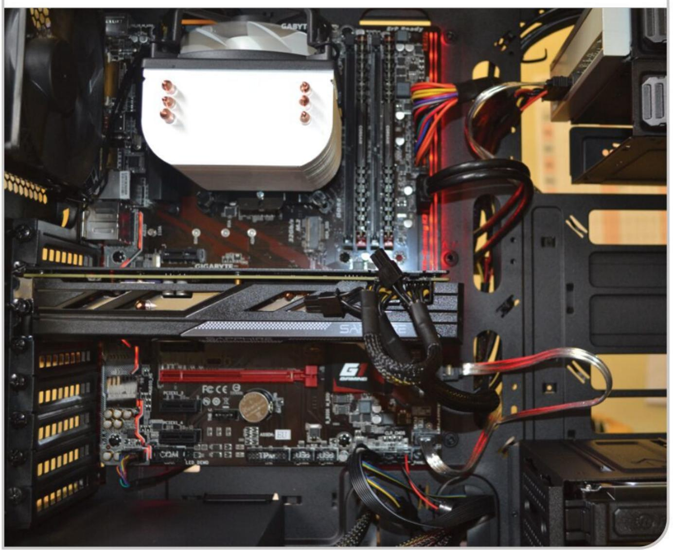
If your case doesn't provide the sort of cable management features we have been talking about here, don't worry, you can still manage the cables. Planning is even more important, as you want as many of the cables as possible running in a single direction. These can then all be gathered together into a bundle, tied up and positioned against the side panel if possible. Not ideal but better than no management!
