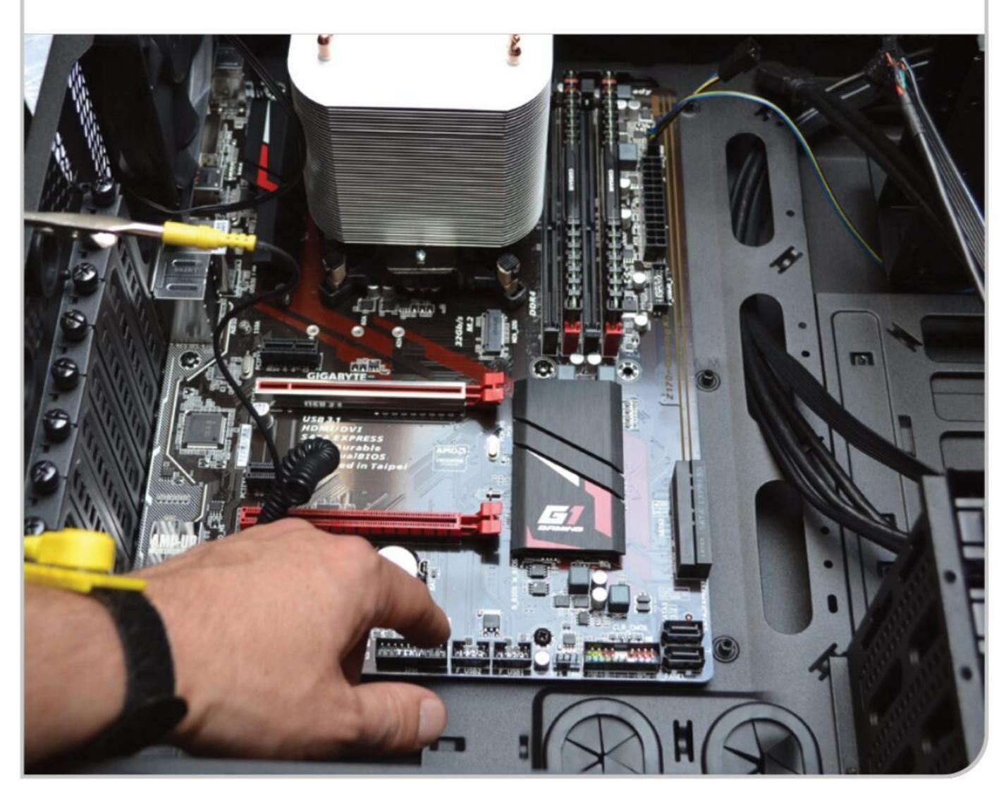
The front USB, audio jacks and case fan connectors are fairly simple to find and connect.
